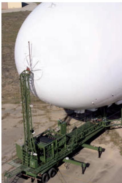
The Aerocraft 3200 mid-size aerostat and relocatable ground mooring station.
